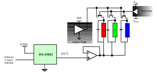
FIGURE 4. DCP SOFTWARE PROGRAMMABLE VCOM IMPLEMENTATION
