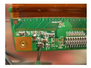
FIGURE 3. ADJUSTMENT OF POTENTIOMETER TO REDUCE FLICKER
